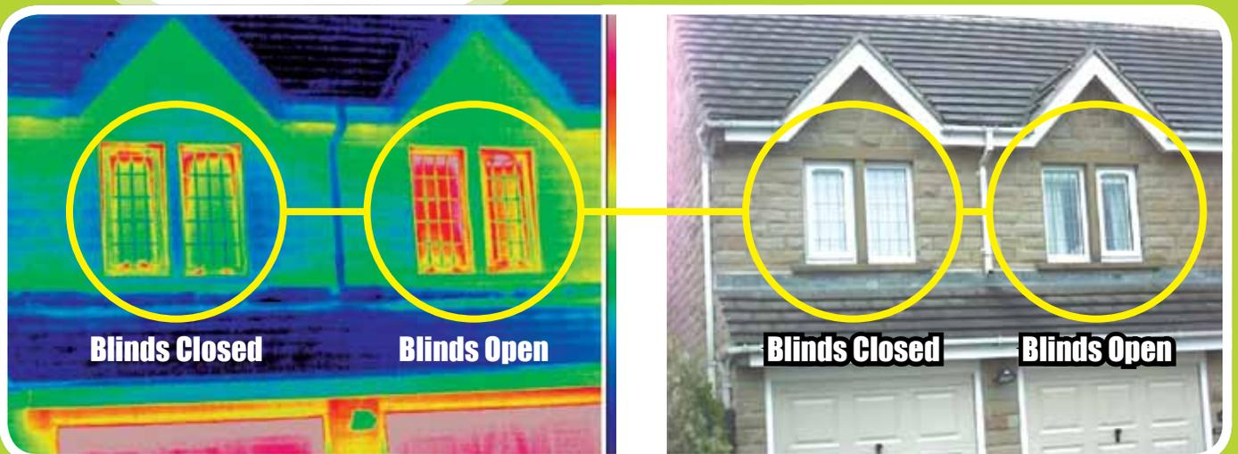
Using a thermal imaging camera you can see the heat loss through the windows without blinds. Red areas correspond to the heat loss.
